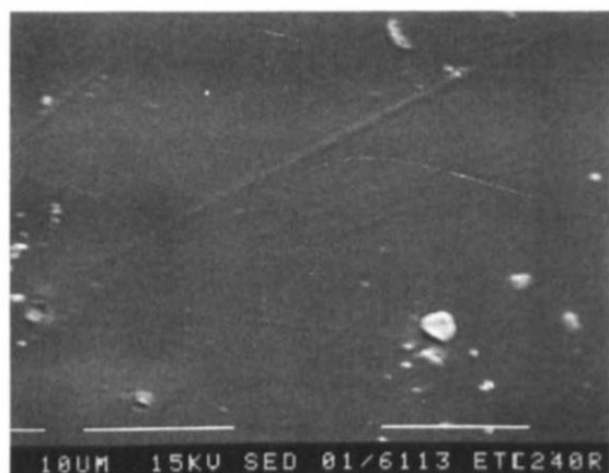
Fig. 2. Scanning electron micrograph of ethylcellulose film prepared by solvent casting (ethanol:toluene (20:80)). Non-porous reverse surface view (3000 \times ).
